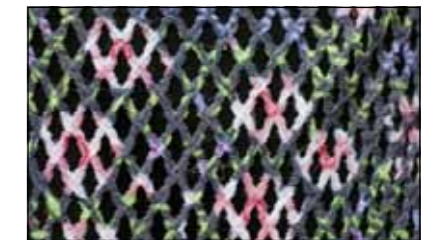
Printed Net Material: Polyester and elastane Application: Hosiery Notes: Complex and intricate patterns are reproduced by transfer printing.
