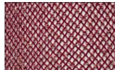
Novelty Yarn Material: Wool, nylon and elastane Application: Hosiery Notes: Novelty yarns are incorporated in the knitted structure to create a unique look and feel.
