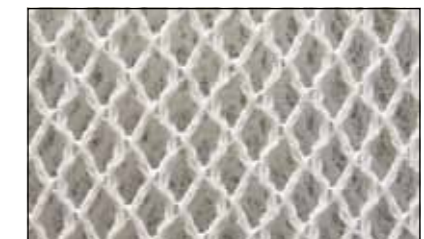
Spacer Textile Material: PP Application: Upholstery Notes: A double-faced diamond net structure is held together by spacer yarns to produce a cushioning fabric.
