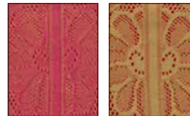
Technical face Technical back Two-Colour Raschel Jacquard Material: Polyester, nylon and elastane Application: Sportswear Notes: Two types of yarn are jacquard knitted and plated to either bring the colour to the front, or hide it inside.
